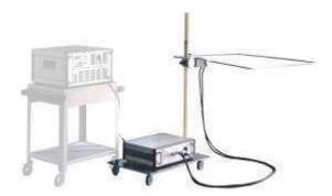
MAG 100 current transformer, 1mx1m antenna mounted on support stand (right) shown with the power source (left)
