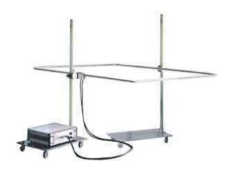
The increased antenna size means that objects up of 1.2m x 1.6m can be tested. However, because the coil antenna is still used with the MAG 100 current transformer, maximum current in the coil is 120A. This results in a magnetic field of only 36A/m at coil center.
